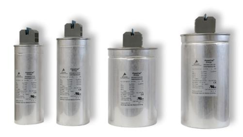
MKK ENERGY capacitors are made by self-healing metallized polypropylene film with very low losses and their can is made by aluminum. The protection from any issue is given by the overpressure disconnector. Three inner overlying capacitances are connected in delta configuration or star configuration in order to reach a high reliabilty during the working cycle. Their construction and tests comply with EN 60831-1/2 (DIN VDE 0560/46).
